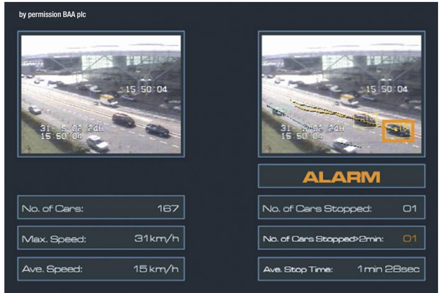
Vehicle counting and stationary vehicle detection and warning alarm.
